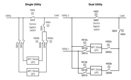
In a redundant system one UPS may be isolated for service/maintenance without affecting other parallel UPS(S).
